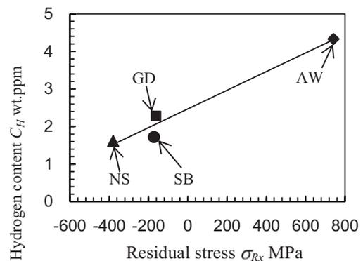
Fig. 8 Increase in hydrogen content along with increase in residual stress
