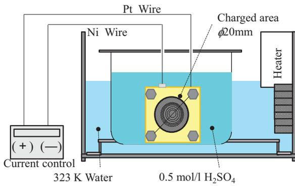
Fig. 1 Apparatus for the cathodic hydrogen charging
