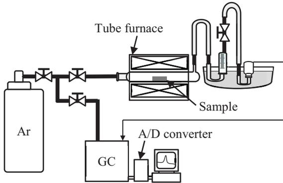
Fig. 4 Apparatus for the thermal desorption analysis
