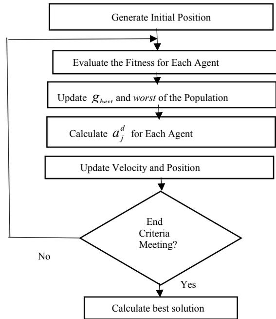
Fig. 2 Flow Chart of Gravitational Search Algorithm
