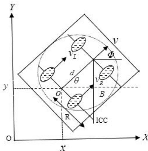
Fig. 1 (a) Four wheeled mobile robot configuration
