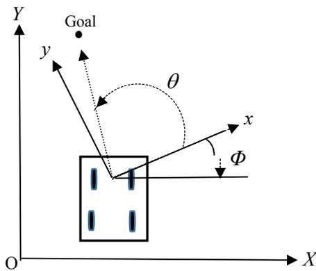
Fig. 1 (b) Robot pose in global coordinates
