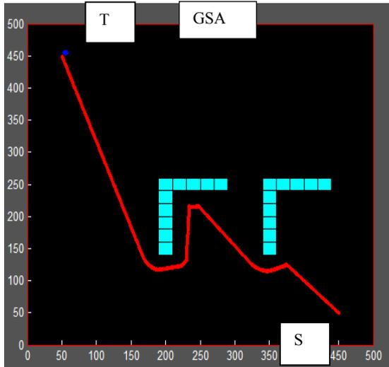
Fig. 6 (a) Robot Start Point (450, 50), Target (50,450)
