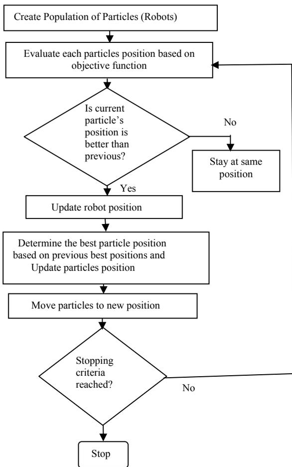
Fig. 5 Flow Chart of Particle Swarm Optimization Algorithm
