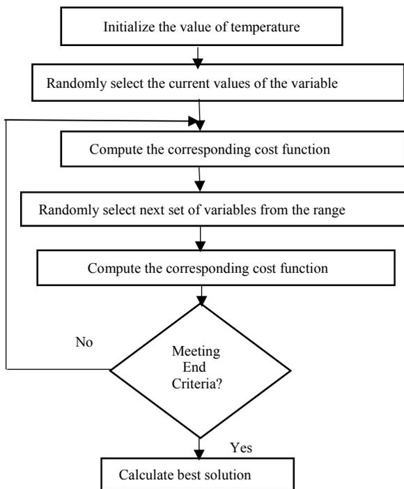
Fig. 3 Flow Chart of Simulated Annealing Algorithm
