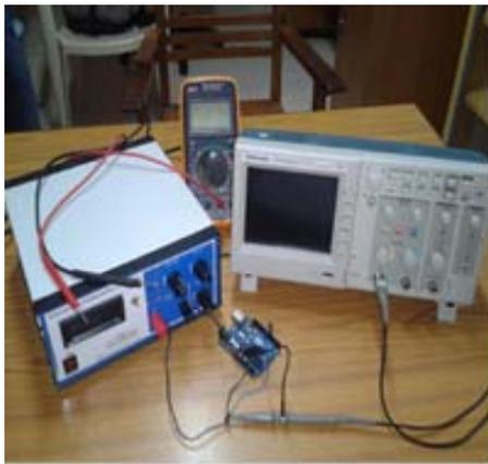
Fig. 9 (b) Testing set up of Arduino Mega 2560
