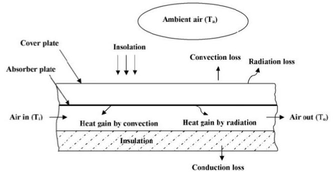
Fig. 1 Energy balance of solar air heater [16]
