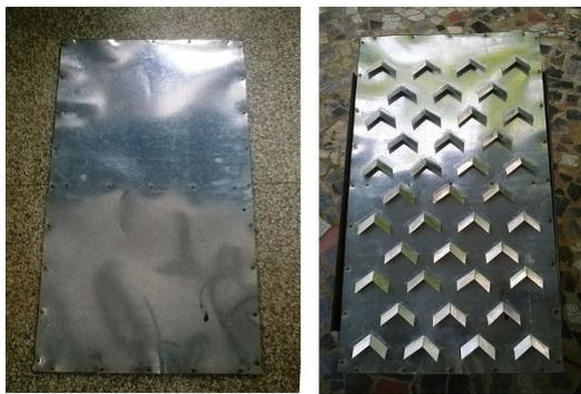
Fig. 3 Smooth and roughened absorber plate
