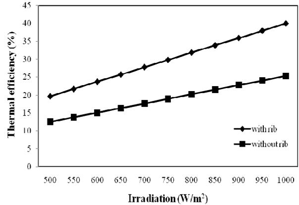
Fig. 4 Variation of thermal efficiency with respect to irradiation
