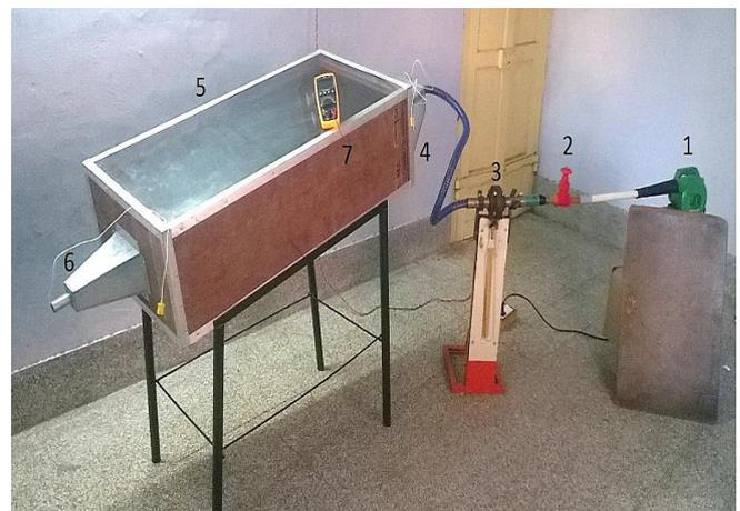
Fig. 2 Experimental setup of solar air collector system
