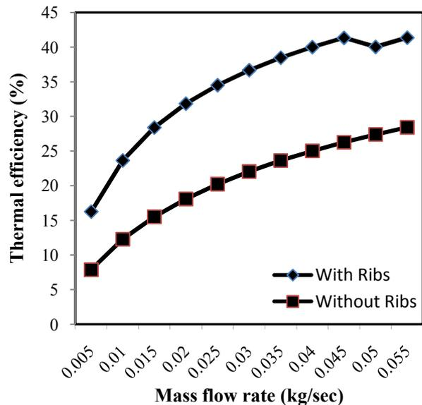
Fig. 5 Variation of thermal efficiency with respect to mass flow rate of air
