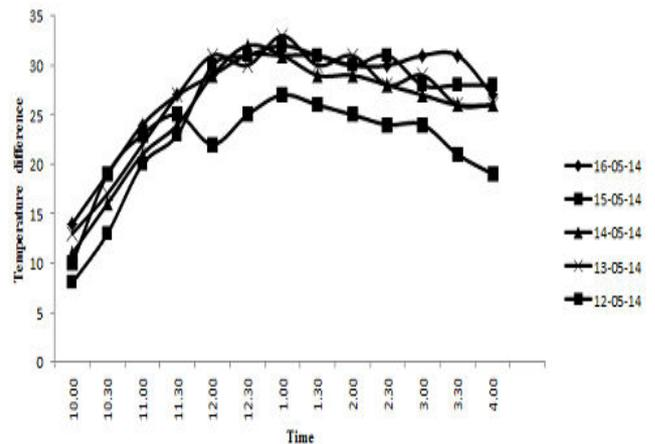
Fig. 9 Variation of temperature in rough solar collector with respect to time
