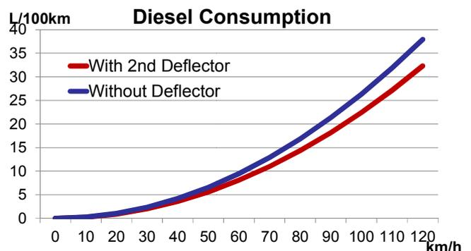
Fig. 6 Diesel consumption at 120 km/h for the configurations with and without the 2<sup>nd</sup> deflector model
