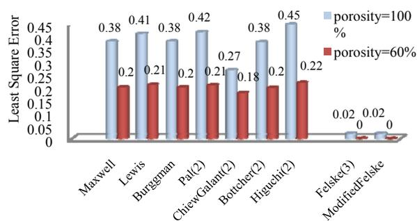
Fig. 8 Comparing error percentage of exist model with improved model with J coefficient for O<sub>2</sub> separation of O<sub>2</sub>/N<sub>2</sub> in PVAC/Zeolit4A
