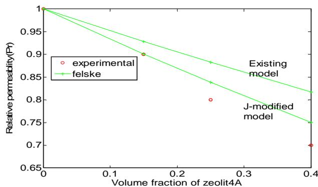
Fig. 4 Comparison of relative permeability O<sub>2</sub> of O<sub>2</sub>/N<sub>2</sub> composition at PVAC/Zeolit4A of existing three-phase models and J-modified models with 60% porosity
