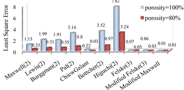
Fig. 6 Comparing error percentage of exist model with improved model with J coefficient for O<sub>2</sub> separation of O<sub>2</sub>/N<sub>2</sub> in Matrimid/CMS
