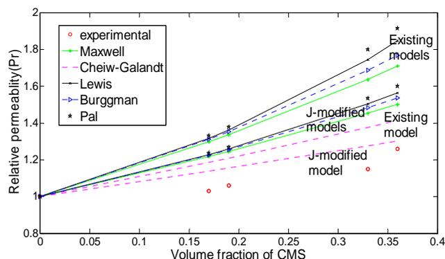
Fig. 3 Comparison of relative permeability CO<sub>2</sub> of CO<sub>2</sub>/CH<sub>4</sub> composition at Matrimid/CMS of existing two-phase models and J-modified models with 80% porosity
