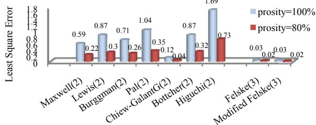
Fig. 5 Comparing error percentage of exist model with improved model with J coefficient for CO<sub>2</sub> separation of CO<sub>2</sub>/CH<sub>4</sub> in Matrimid/CMS
