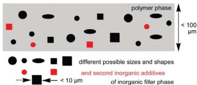
Fig. 2 Schematic of a mixed-matrix membrane [9]
