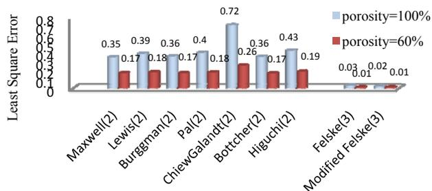
Fig. 7 Comparing error percentage of exist model with improved model with J coefficient for O<sub>2</sub> separation of O<sub>2</sub>/N<sub>2</sub> in BAPD-BPADA/Zeolit4A
