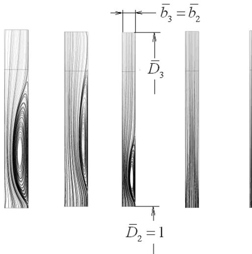
Fig. 3 Meridian streamlines in diffusers with different width at different inlet angles. From left to right:  $\bar{b}_2 = 0,10$ ,  $\alpha_2 = 10$  and  $20^\circ$ ,  $\bar{b}_2 = 0,057$ ,  $\alpha_2 = 10^\circ$ ,  $\bar{b}_2 = 0,014$ ,  $\alpha_2 = 10^\circ$ ,  $\lambda_{c2} = 0,64$ ,  $Re_{D2} = 9,1E+6$
