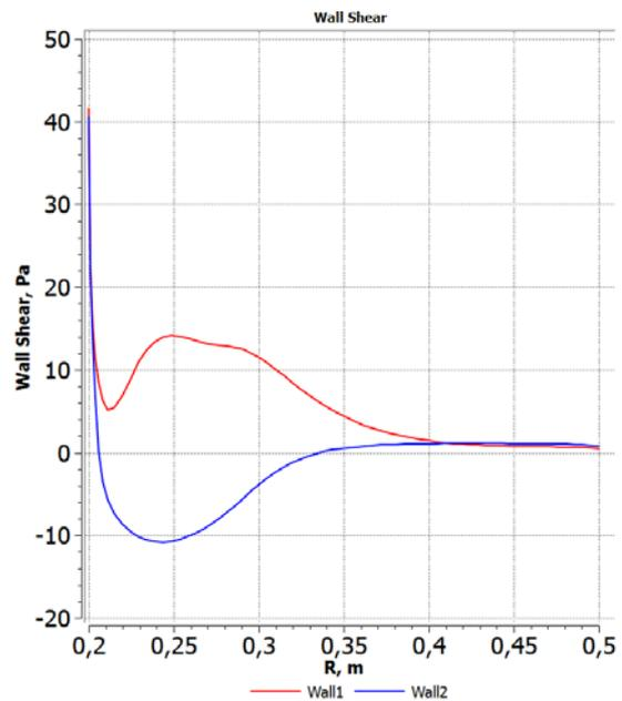
Fig. 4 Shear stress radial component at walls of the diffuser:  $\bar{b}_2 = 0,057$ ,  $\alpha_2 = 10^\circ$ ,  $\lambda_{c2} = 0,64$ ,  $Re_{D2} = 9,1E6$
