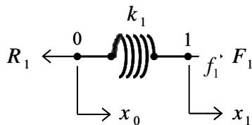
Fig. 4(a) Boundary condition of spring-1
