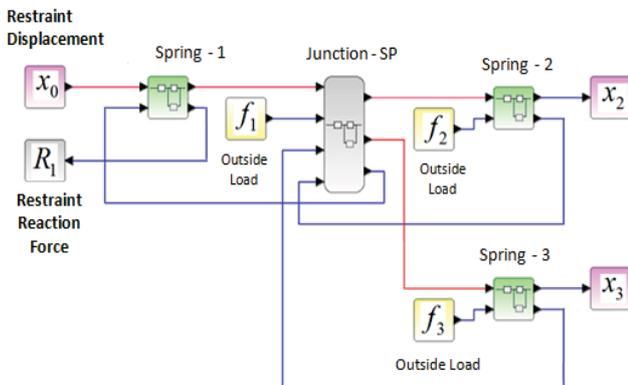
Fig. 8 Model diagram in semi-causal modeling
