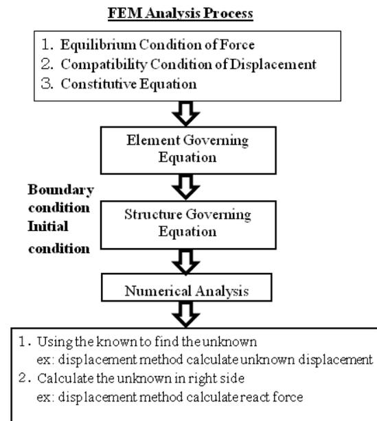
Fig. 3 (b) Outline procedure of FEM analysis diagram
