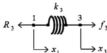
Fig. 4(c) Boundary condition of spring-3
