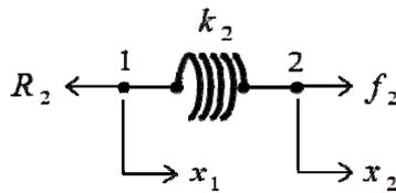
Fig. 4(b) Boundary condition of spring-2
