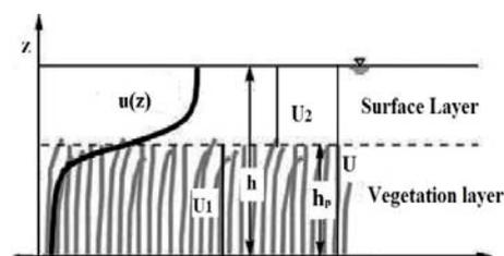
Fig. 1 Velocity profile within and above vegetation
