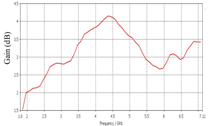
Fig. 7 The proposed antenna gain versus frequency
