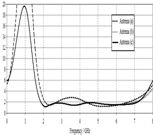
Fig. 4 The VSWR of the three antenna structures
