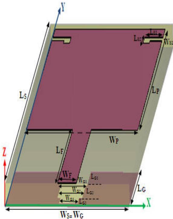
Fig. 1 Perspective view of the proposed antenna
