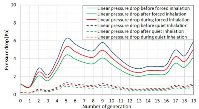
Fig. 13 Linear pressure drop in the airways during quit and forced inhalation
