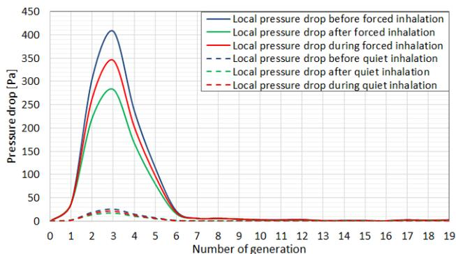
Fig. 11 Local pressure drop in the airways during quit and forced inhalation
