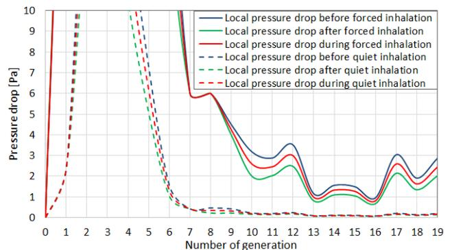
Fig. 12 Local pressure drop in the airways during quit and forced inhalation - detail the terminal bronchiole
