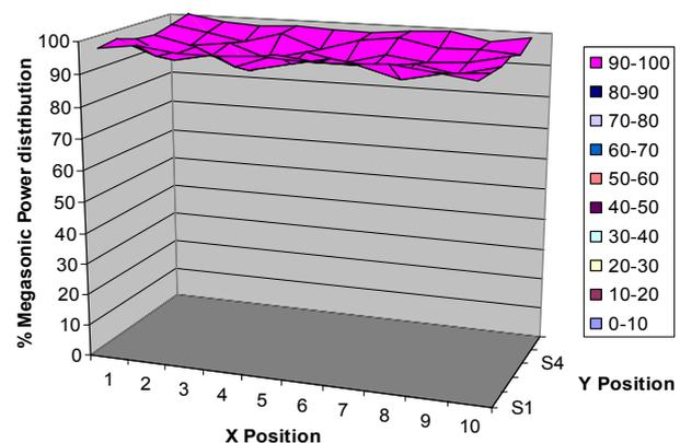
Fig. 3 Megasonic sweeping power distribution pattern in a cleaning vessel for 360 kHz
