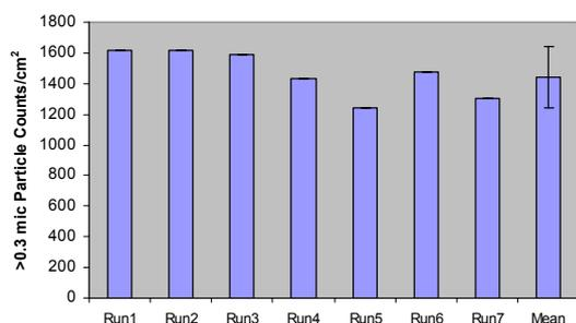
Fig. 6 Run to run cleaning variation for aluminum metal spacer
