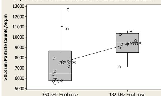
Fig. 10 Particle retain after washing aluminum metal spacer
