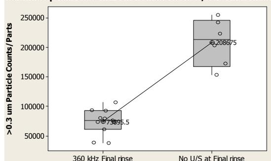
Fig. 9 Particle retain after washing for ceramic spacer
