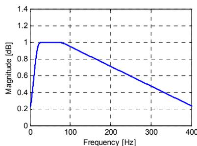
Fig. 5 IIR filter Yule-Walk frequency response gain
