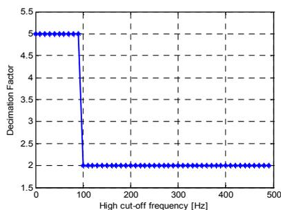
Fig. 2 Evolution of decimation factor with fault frequency
