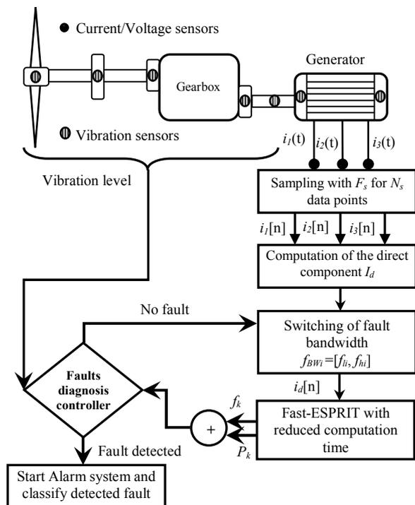
Fig. 3 Intelligent wind turbine faults diagnosis by Fast-ESPRIT
