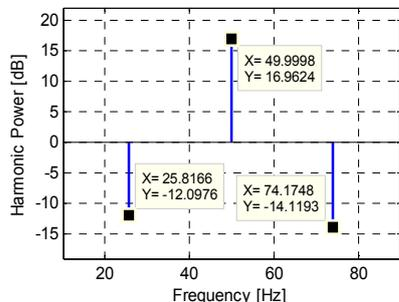
Fig. 6 Power and Frequency estimates by Fast-ESPRIT for eccentricity fault
