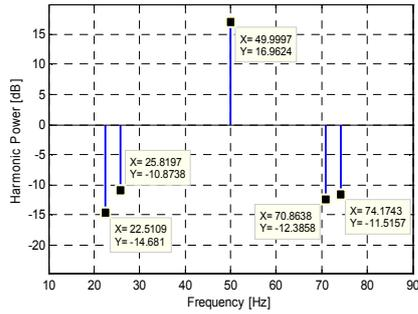
Fig. 10 Power and Frequency estimates by Fast-ESPRIT for broken rotor bars fault
