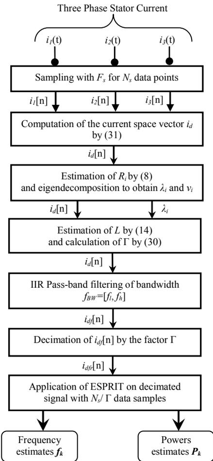
Fig. 1 Block diagram scheme of the Fast-ESPRIT algorithm
