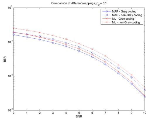
Fig. 2 Comparison of ML and MAP detection
