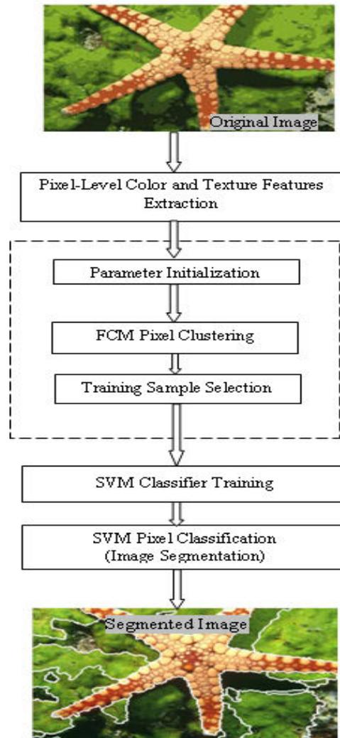
Fig. 3 Image Segmentation using SVM Pixel Classification
