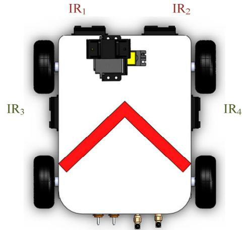
Fig. 5 IR sensors location on the AMR
