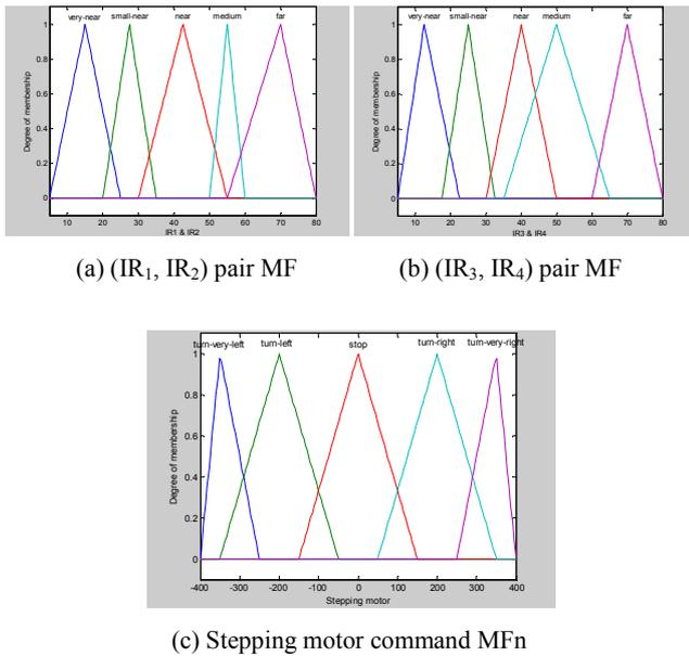
Fig. 7 Type II fuzzy controller obstacle avoidance mode
