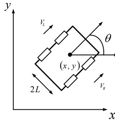
Fig. 1 Kinematic model of a mobile robot
