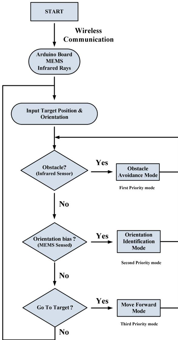
Fig. 4 Hybrid control mode for autonomous mobile robot
