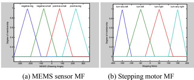
Fig. 8 Type I fuzzy controller for orientation identification mode
