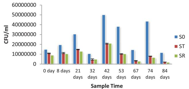
Fig. 14 Change in CFU/ml during treatment by HSSF mesocosms planted with *Typha* and *Ranunculus*
