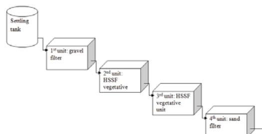
Fig. 1 Schematic representation of HSSF mesocosms
