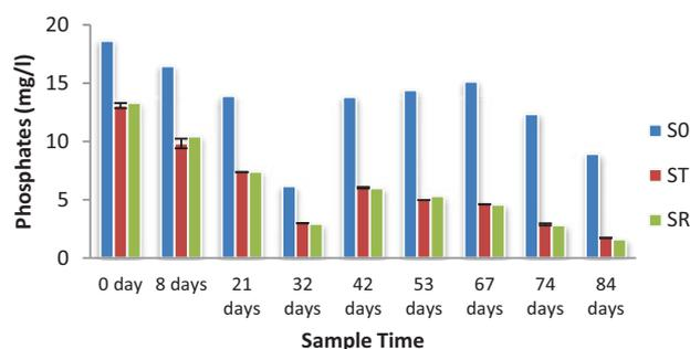
Fig. 10 Change in Phosphates concentration during treatment by HSSF mesocosms planted with *Typha* and *Ranunculus*
