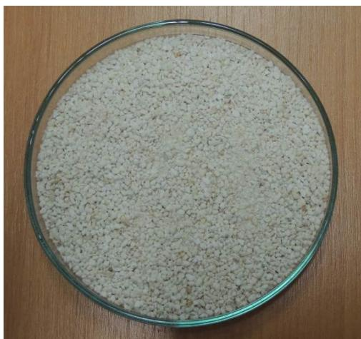
Fig. 1 Demonstration aggregates derived from volcanic glass
