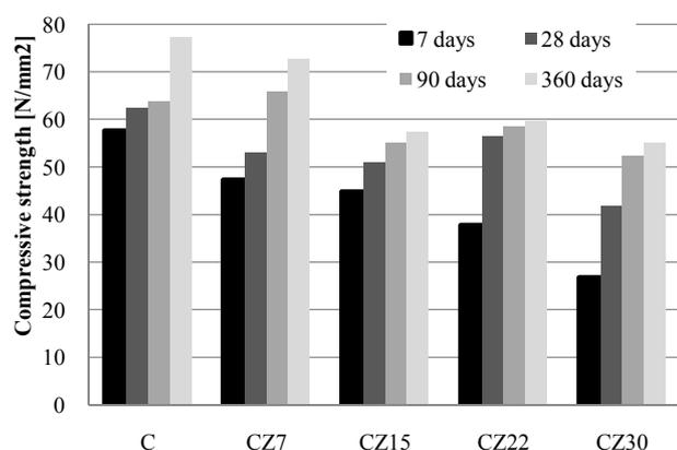
Fig. 3 Compressive strength after 7, 28, 90 and 360 days
