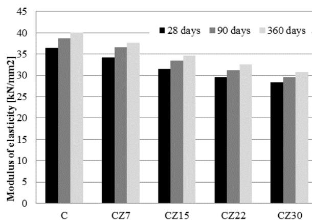
Fig. 4 Modulus of elasticity after 7, 28, 90 and 360 days
