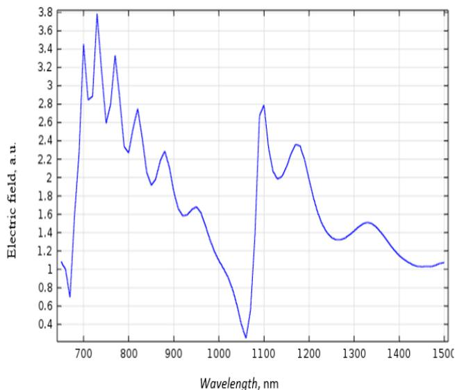
Fig. 3 (b) Near-field Electric field component spectrum
