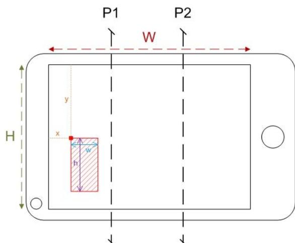
Fig. 5 Determination of the relative object's position
