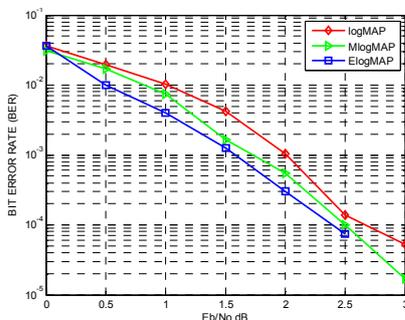
Fig. 6 Performance of decoding algorithms for class 1 in fading channel
