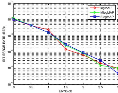
Fig. 5 Comparison of Turbo decoding algorithms for class 3 in AWGN Channel
