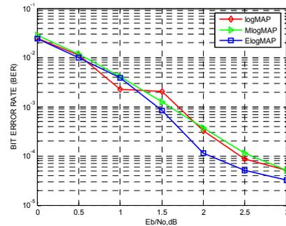
Fig. 3 Comparison of Turbo decoding algorithms for class 1 in AWGN Channel
