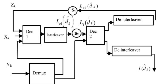
Fig. 1 Turbo Decoder with Double Scaling factor
