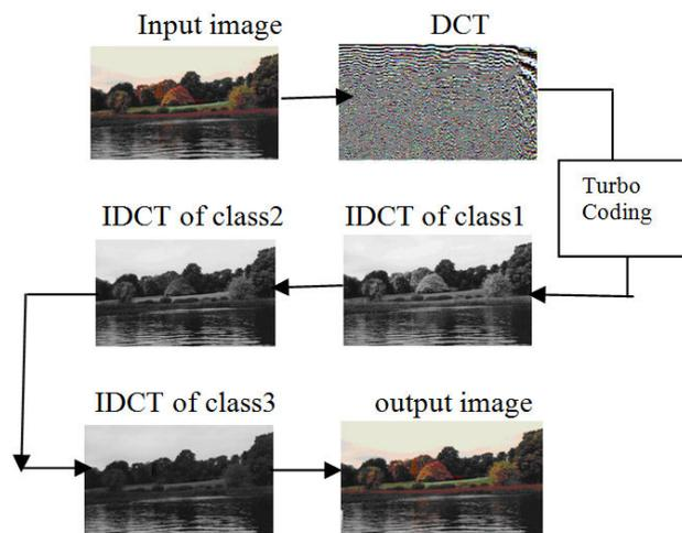
Fig. 12 Image transmission and retrieval using JSCC
