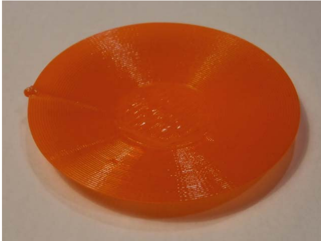
Fig. 14 Printed plate with 15° gradient round using Slic3r (layer height: 0.135 mm)
