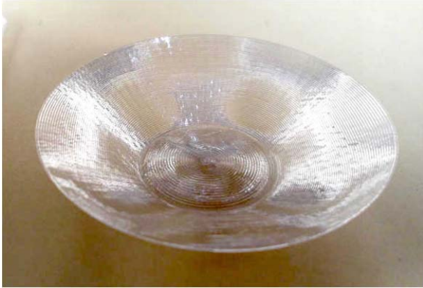
Fig. 3 A small plate printed by the helical/spiral printing method
