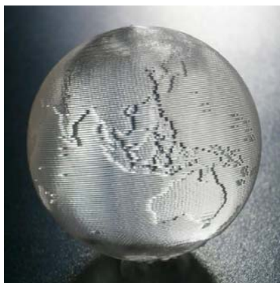
Fig. 4 A small globe printed by the helical/spiral printing method
