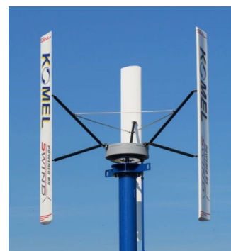
Fig. 8 VAWT wind plant with Komel's generator
