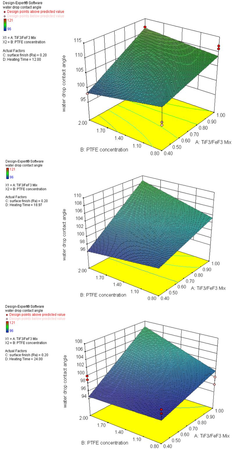
Fig. 6 DOE Response surface Model (RSM) of water drop contact angle for 0.2  $\mu\text{m}$   $R_a$  surface roughness with respect to different heating time of the lubricant at 100°C, different PTFE % concentration and different  $\text{TiF}_3/\text{FeF}_3$  catalysts % concentration.
