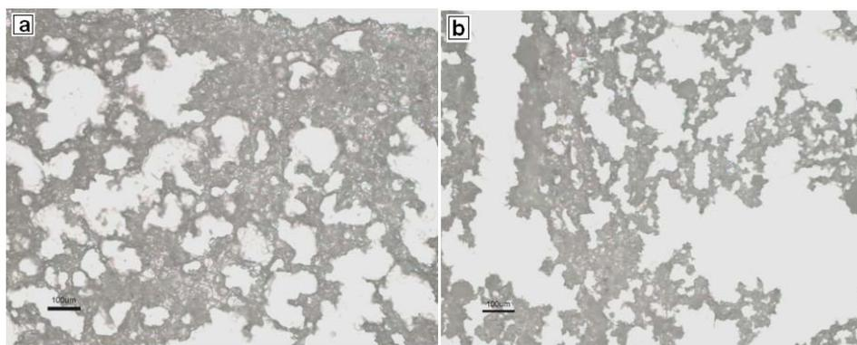
Fig. 7 Scanning Electron Micrograph of PTFE/TiF<sub>3</sub>/FeF<sub>3</sub> deposition on 0.1 μm R<sub>a</sub> surface roughness (a) and on 0.05 μm R<sub>a</sub> surface roughness (b). Bearing steel surfaces were treated for 24 hours at 100°C in 0.05 P % ZDDP + 0.5 wt. % TiF<sub>3</sub> + 0.5 wt. % FeF<sub>3</sub> + 2 wt. % PTFE and the balance 100-neutral base oil
