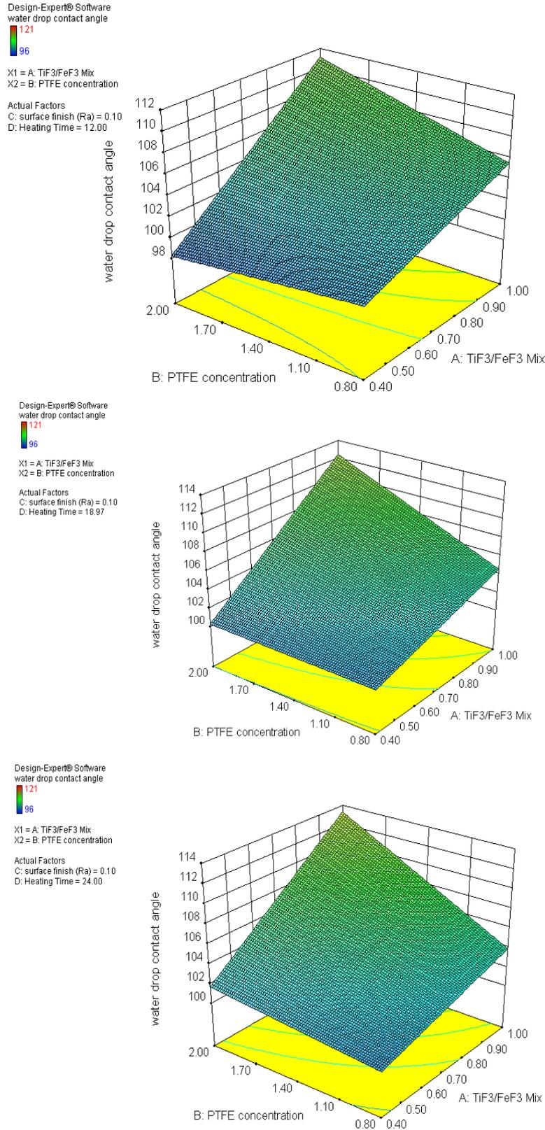
Fig. 5 DOE Response surface Model (RSM) of water drop contact angle for 0.1  $\mu\text{m}$   $R_a$  surface roughness with respect to different heating time of the lubricant at 100°C, different PTFE % concentration and different TiF<sub>3</sub>/FeF<sub>3</sub> catalysts % concentration
