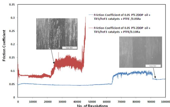
Fig. 8 Tribological behavior of two surface finishes treated with 0.05 P % ZDDP + 0.5 wt. % TiF<sub>3</sub> + 0.5 wt. % FeF<sub>3</sub> + 2 wt. % PTFE and the balance 100-neutral base oil for 24 hours at 100°C under an extreme load of 336 Newton or 2.6 GPa Hertzian pressure
