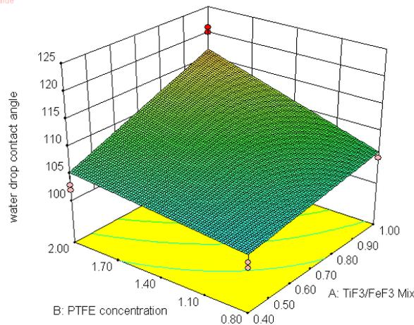
Fig. 4 DOE Response surface Model (RSM) of water drop contact angle for 0.05 μm R<sub>a</sub> surface roughness with respect to different heating time of the lubricant at 100°C, different PTFE % concentration and different TiF<sub>3</sub>/FeF<sub>3</sub> catalysts % concentration.
