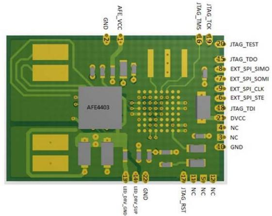
Fig. 4 Rendered PCB of the developed monitoring device
