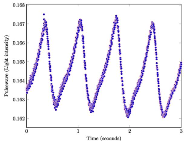
Fig. 6 PPG signal, measured by experimental device
