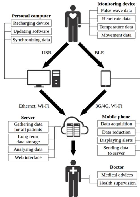
Fig. 1 Structure and functions of health monitoring system
