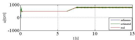
Fig. 1 Real and estimated speed in acceleration test
