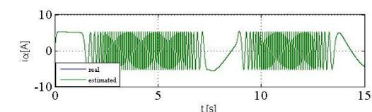
Fig. 4 Real and estimated current components in speed inversion test
