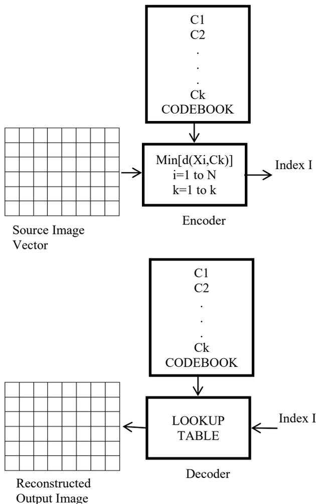
Fig. 2 Basic block diagram of vector quantization
