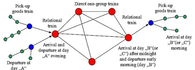
Fig. 3 Implementation of time-discrete train formation technology
