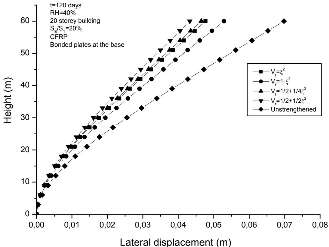
Fig. 1 Effect of the fibers distribution on the lateral displacement of shear wall strengthened
