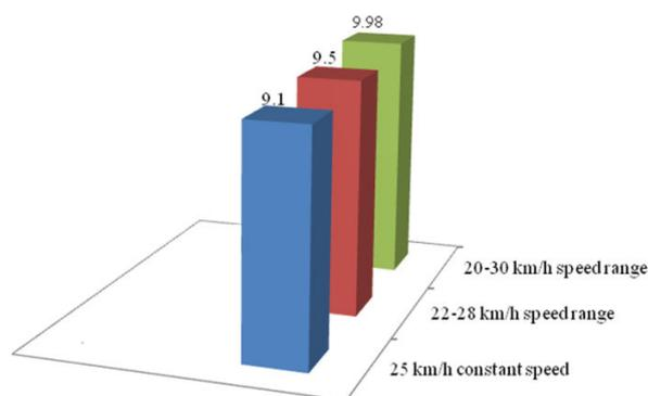
Fig. 6 Hydrogen consumption for three driving strategies (l/min)
