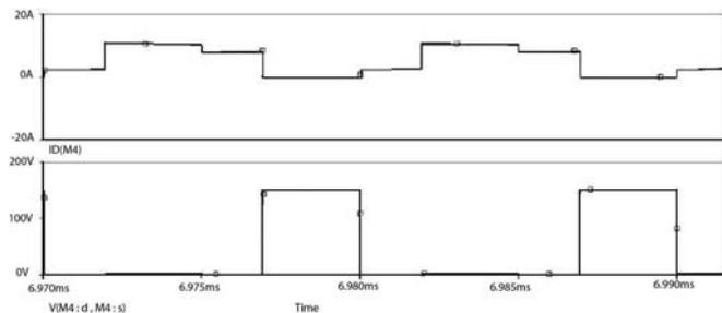
Fig. 5 Voltage and current stresses of flyback based converter
