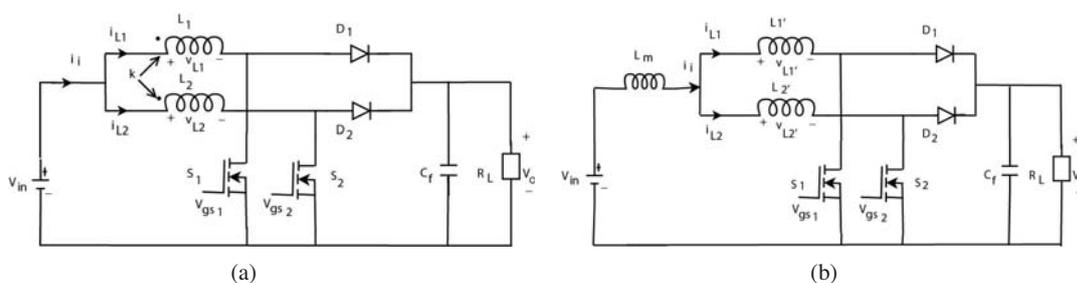
Fig. 2 (a) Interleaved boost converter (b) Equivalent circuit of the interleaved boost converter. ( $i_i$ : input current,  $L$ : coupled inductor,  $L'$ : uncoupled inductor,  $i_L$ : inductor current,  $L_m$ : mutual inductor,  $V_L$ : inductor voltage,  $D$ : diode,  $V_{in}$ : input voltage,  $S_1$  and  $S_2$ : active switches,  $V_{gs1}$  and  $V_{gs2}$ : controlled signals for active switches,  $C_f$ : output filter capacitance,  $R_L$ : load resistance, and  $V_o$ : output voltage)
