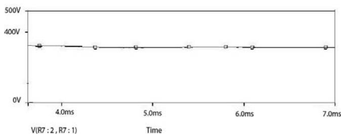
Fig. 3 Output voltage of flyback based converter
