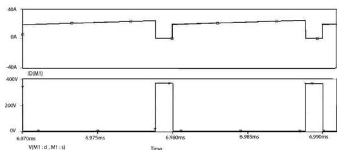
Fig. 11 Voltage and current stresses of boost converter
