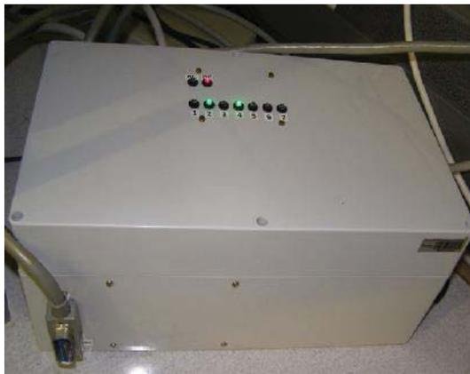
Fig. 4 Programmable GPIB switching isolator (up to 7 channels)
