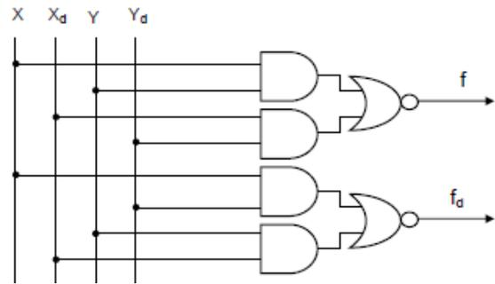
Fig. 2 Dual rail checker cell
