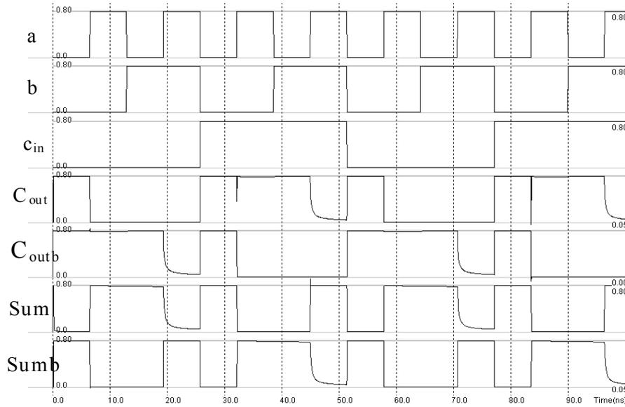
Fig. 4 SPICE simulation of the adder in 32nm DPL technology with injection of primary fault ( $a = \bar{a}$ )
