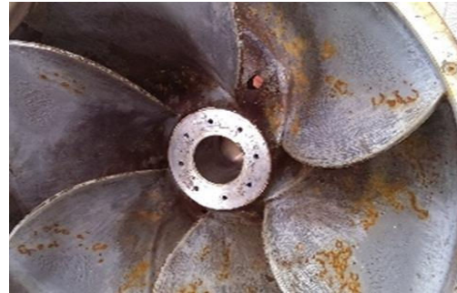
Fig. 16 Cavitation of Impeller
