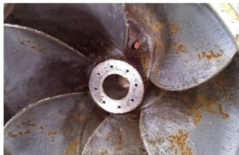
Fig. 16 Cavitation of Impeller
