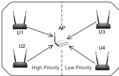
Fig. 4 A star-topology WLAN with priority for WT2F [5]
