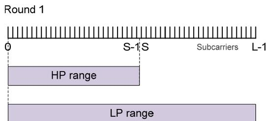
Fig. 5 HP and LP subcarrier ranges for WT2F [5]
