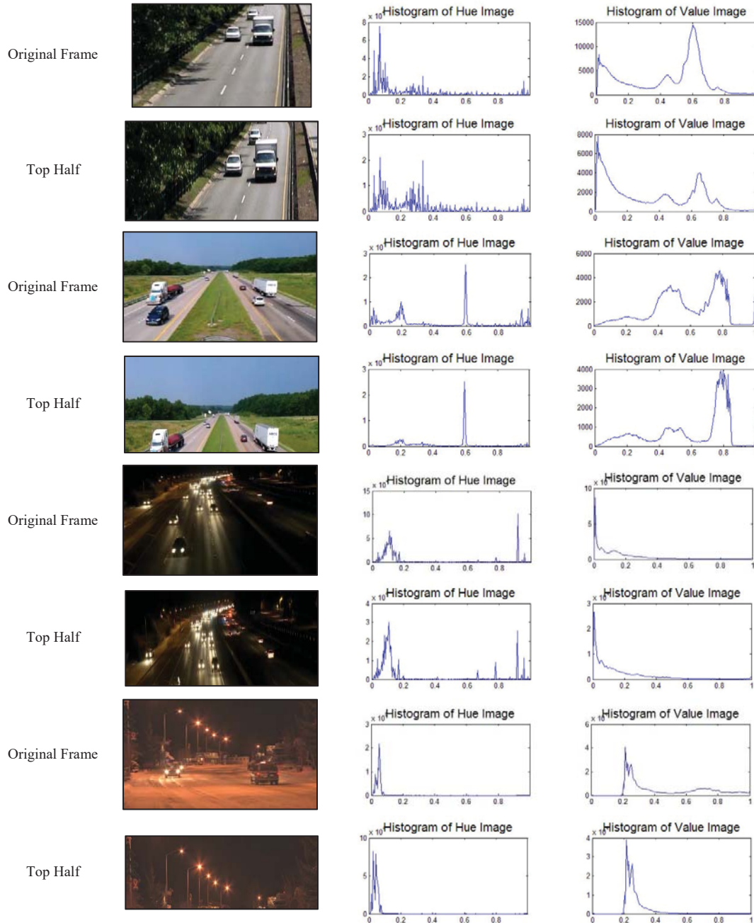
Fig. 1 Comparative H-Histogram & V-Histogram of original frame and its top half image for different daytime / nighttime traffic videos
