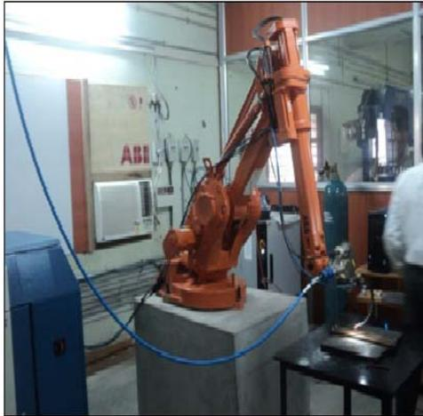
Fig. 5 Nd:YAG laser welding system
