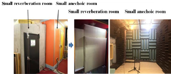
Fig. 3 Small reverberation room and small anechoic room
