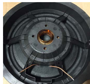
Fig. 1 Loudspeaker only the vibration system
