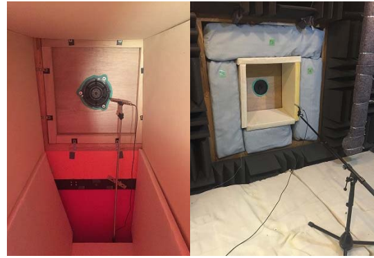
Fig. 6 Reverberation room and anechoic room
