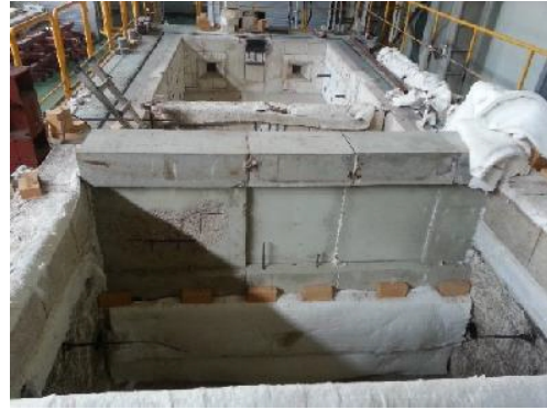
Fig. 2 Specimens placed in horizontal heating chamber
