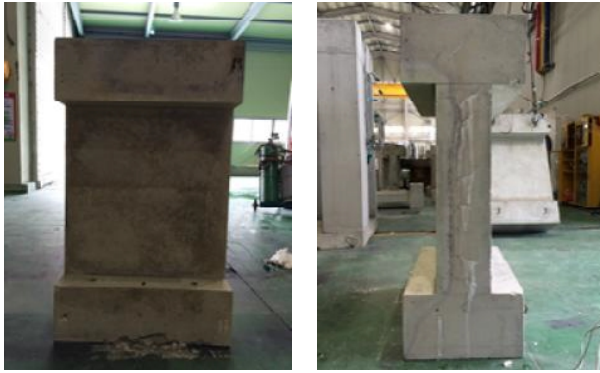
Fig. 5 Specimen after heated for 2 hours
