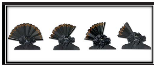
Fig. 6 Movement of the fan with the help of servo motor attached to the neckline which reacts to the proximity sensor
