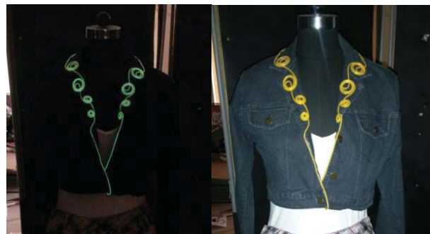
Fig. 9 Denim jacket embedded with EL wire in synchronization to music, thus allowing multiple lengths of EL wire to be flashed in a desired sequence
