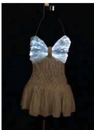
Fig. 3 Interactive garment with the torso made of Polymeric optical fiber fabric that gives a rhythmic display of lights reacting to music
