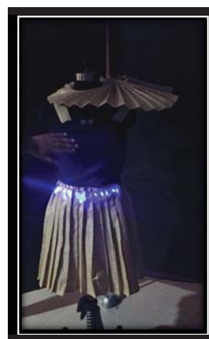
Fig. 5 Pleated skirt Interactive garment integrated with proximity sensors, servomotor and LED's
