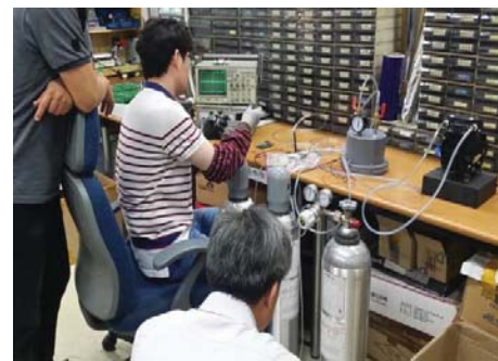
Fig. 4 Performance test of a prototype ammonia detector
