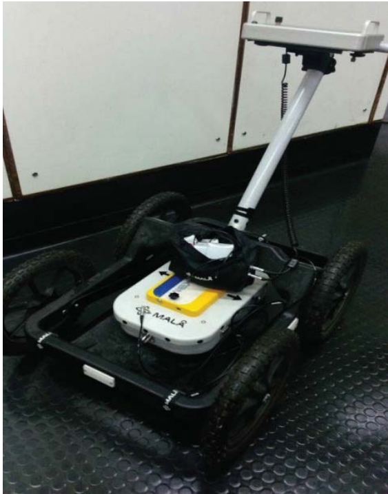
Fig. 1 GPR on a Terraplus Rough Terrain Cart
