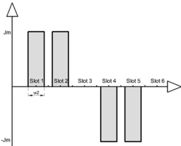
Fig. 3 Distribution of stator slots current density
