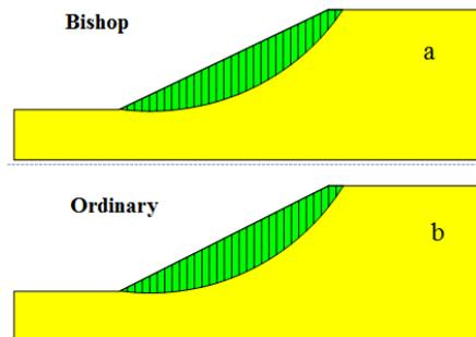
Fig. 3 Slip surfaces by slices method
