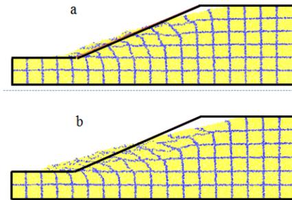
Fig. 2 Deformation of slope by Distinct Element Method
