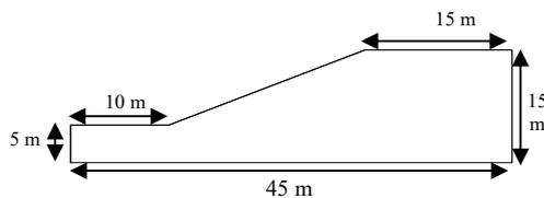
Fig. 1 Slope geometry
