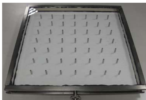
Fig. 9 Fabricated flat vacuum panel
