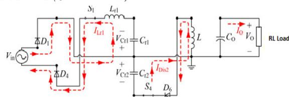
Fig. 5 Equivalent Circuit Diagram of Mode 1
