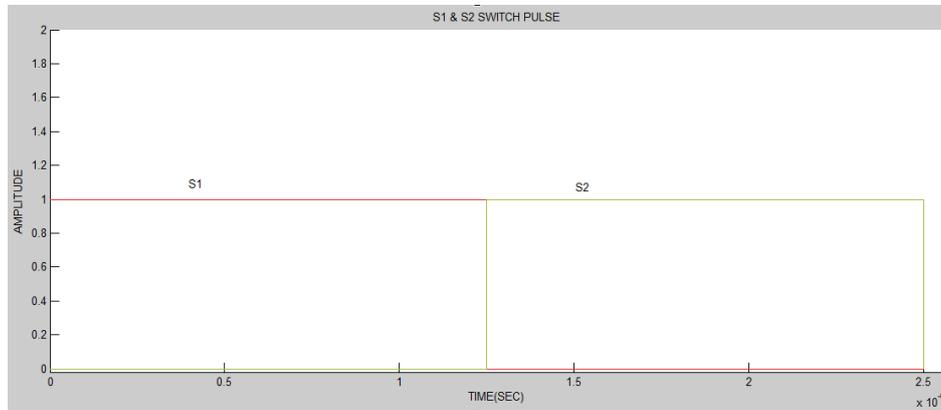
Fig. 9 Gate pulse signals for Switches S1, S2
