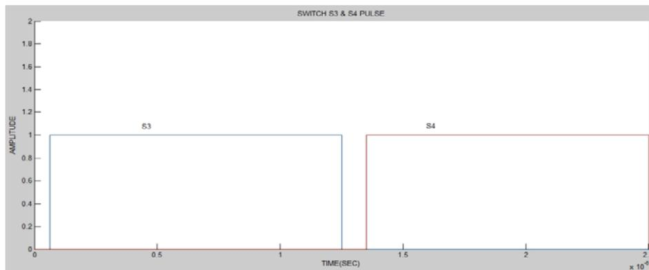
Fig. 10 Gate pulse signals for Switches S3, S4
