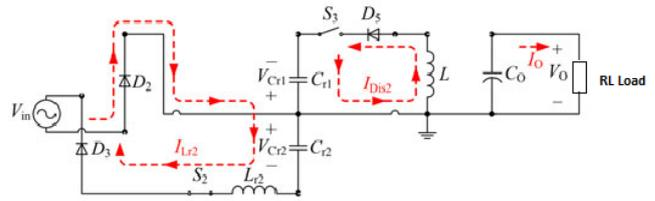
Fig. 7 Equivalent Circuit Diagram of Mode 3
