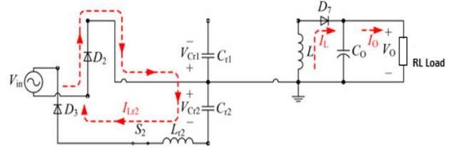
Fig.8 Equivalent Circuit Diagram of Mode 4
