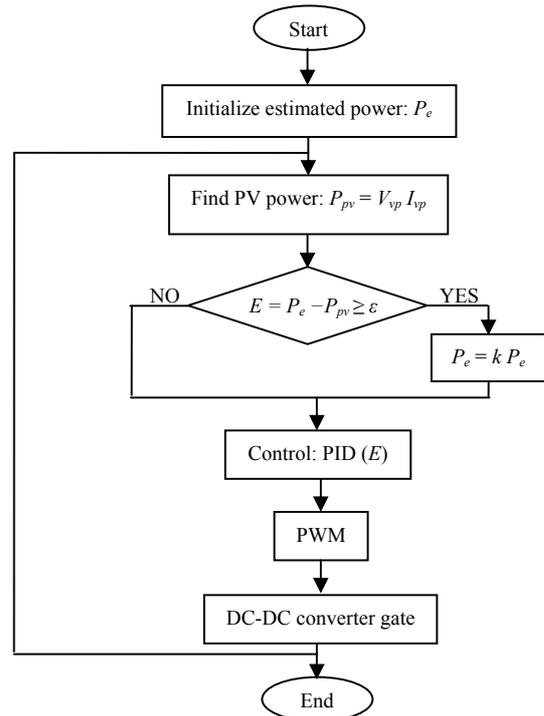
Fig. 6 Flow-chart of the proposed MPPT method
