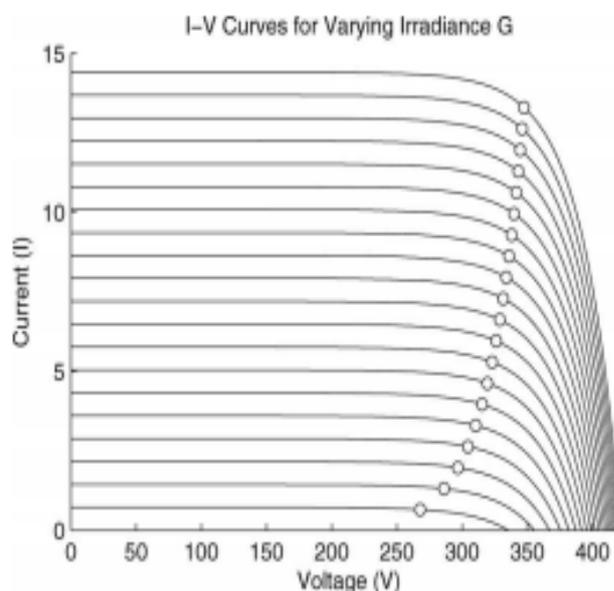
Fig. 3 I-V curves under difference operating conditions
