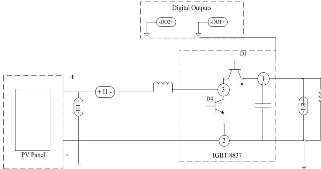
Fig. 5 Configuration of the PV energy conversion system
