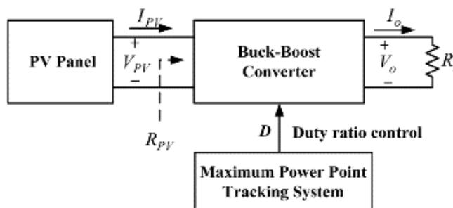
Fig. 4 PV energy conversion system and MPPT
