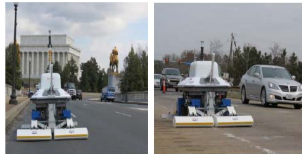
Fig. 3 Operation of GPR bridge deck assessment robot [14]
