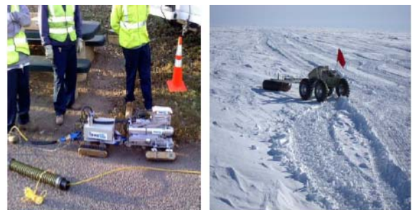
Fig. 4 Sewervue [15] and Yeti Robot [16] in operation
