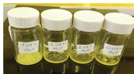
Fig. 2 Photograph of DMF/PbI 2 precursor solutions consisting of various amounts of additive DI-H 2 O
