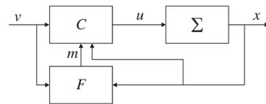
Fig. 1 Corrective control system with a fault detector
